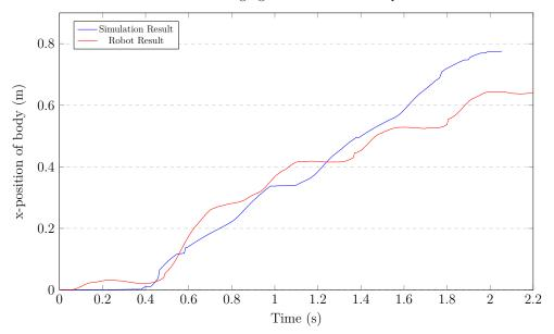
**Figure 6.9:** z- and x-position comparison between the simulated multi-surface trajectory and the robot hopping from a hard surface to rough gravel. The line on the z-Position graph indicate the trigger height for when the pneumatic cylinder goes from contraction to expansion.
