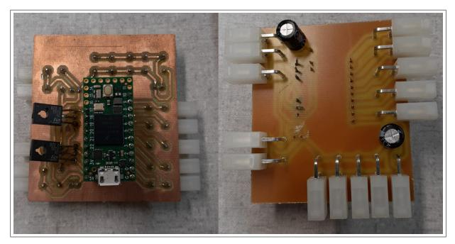
Figure 4.3: Top and bottom view of the designed PCB with the Teensy connected to it.
