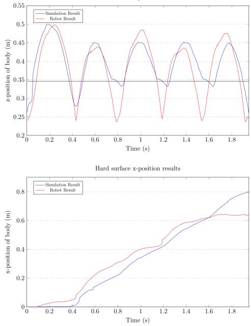
**Figure 6.5:** z- and x-Position comparison between the hard surface trajectory and the free body robot hopping on a hard surface. The line on the z-Position graph indicate the trigger height for when the pneumatic cylinder goes from contraction to expansion.
