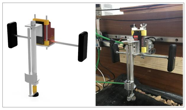
**Figure 4.1:** CAD model of the robot including the linear support rail compared to the fully built robot
