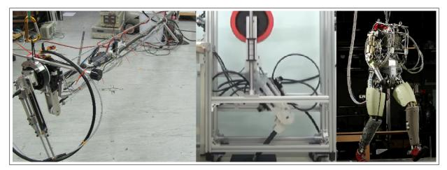
**Figure 2.6:** The different support rigs discussed in this section, on the left is the boom support rig used in [9], in the middle is the support rig used by the Kenji Hashimoto Lab [47] and on the right is an older version of the Atlas robot [26] that is tethered.
