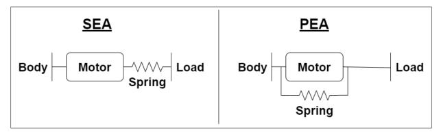
**Figure 2.4:** This figure shows that with SEA the spring is placed between the motor and the load, and with PEA the spring is placed between the body and the load.
