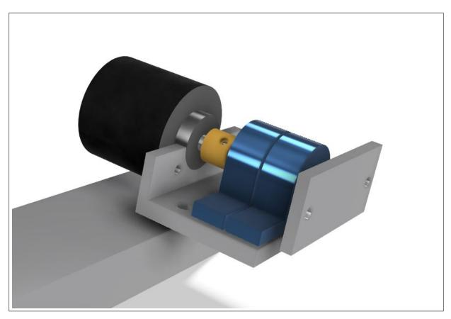
Figure 4.8: Render of the design of the bearing mounts and encoder attachments.
