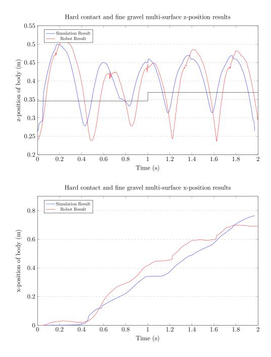
**Figure 6.10:** *z*- and *x*-position comparison between the simulated multi-surface trajectory and the robot hopping from a hard surface to fine gravel. The line on the *z*-Position graph indicate the trigger height for when the pneumatic cylinder goes from contraction to expansion.
