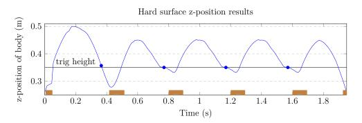
**Figure 6.1:** *z*-Position simulated trajectory with blue dots where the cylinder will go from contraction to expansion. The intermittent brown lines at the bottom of the graph indicate when the foot of the robot touches the ground.
