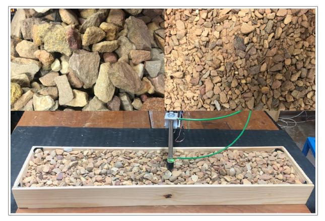
Figure 4.9: Image of gravel pit with robotic platform and the two types of gravel used
