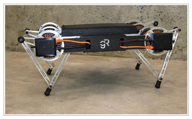
**Figure 2.3:** The Minitaur robot [33] with a clear view of its direct drive motors attached to the legs.
