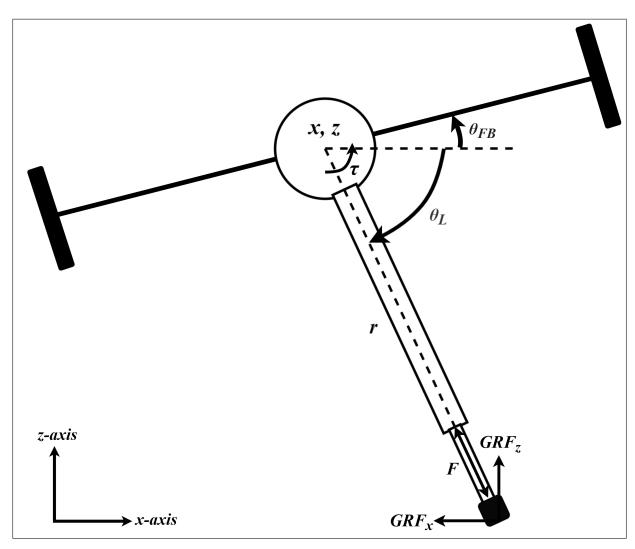
**Figure 3.1:** Model of mono-pod robot showing the generalized coordinates and the basis vectors as well as the applied forces and torques. The black rectangles in the image are the inertial weights added to stabilize the body.
