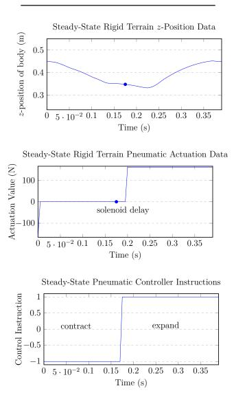
**Figure 6.2:** A rigid terrain steady-steady trajectory with a blue dot on the node where the solenoid needs to be triggered for pneumatic actuation.
