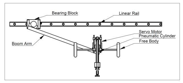
Figure 4.6: Front view drawing of robot platform and free body rig
