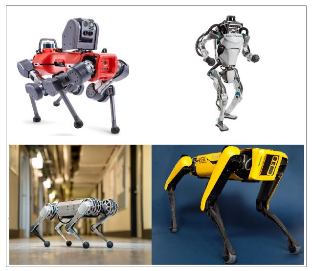
**Figure 2.2:** Top left is the ANYmal robot developed by ETH Zurich [25]. Bottom left is the Mini Cheetah made by MIT [27]. A biped and quadruped developed by Boston Dynamics, Atlas and Spot are shown on the top and bottom right of the figure [26].
