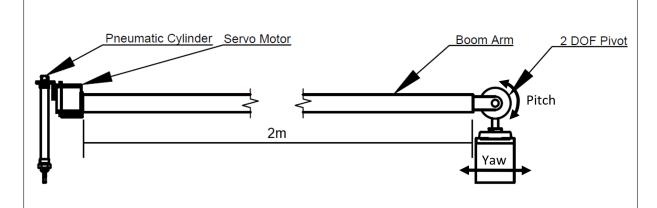
**Figure 4.4:** Side view drawing of robot platform and fixed body rig indicating degrees of freedom and important components
