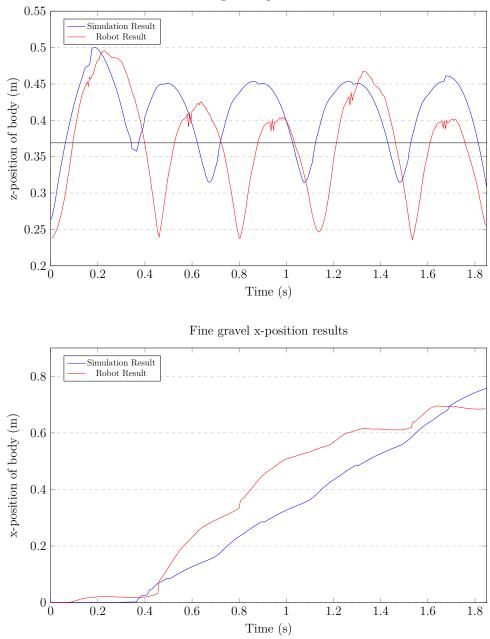
**Figure 6.7:** *z*- and *x*-Position comparison between the fine gravel trajectory and the free body robot hopping on fine gravel. The line on the z-Position graph indicate the trigger height for when the pneumatic cylinder goes from contraction to expansion.
