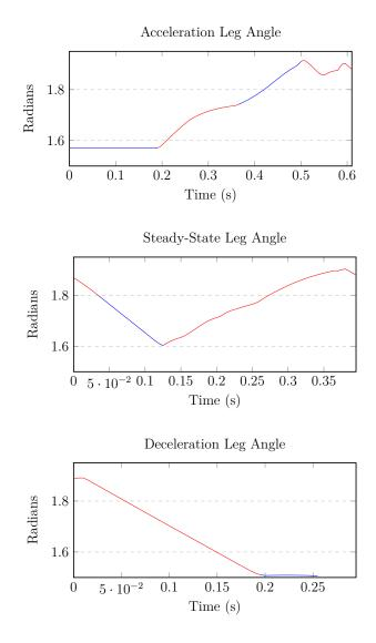
**Figure 6.3:** The change in leg angle for an acceleration, steady-state and deceleration trajectories on rigid terrain. The red indicates that the foot is in the air, and blue indicates that the foot is on the ground.
