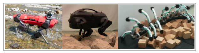
**Figure 2.7:** The robots that tested the different approaches to overcoming rough terrain. ETH Zurich AnyMAL on the left, the littleDog in the middle and the Shinayaka robot on the right.
