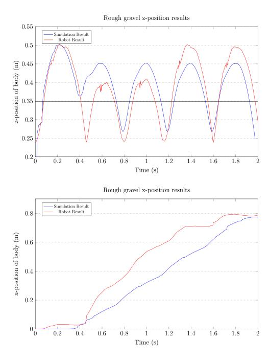
**Figure 6.6:** z- and x-Position comparison between the rough gravel trajectory and the free body robot hopping on rough gravel. The line on the z-Position graph indicate the trigger height for when the pneumatic cylinder goes from contraction to expansion.
