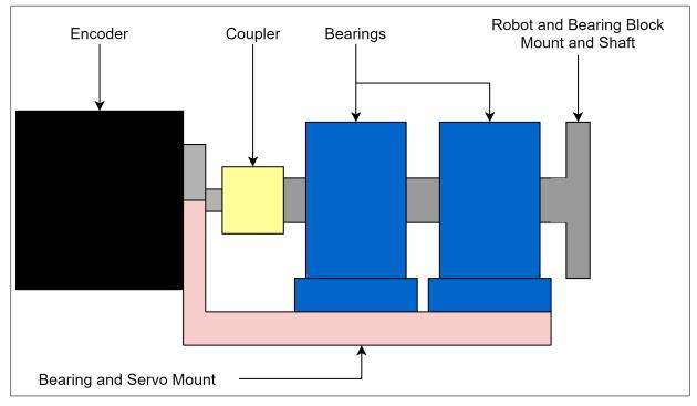
Figure 4.7: Side view of encoder and bearing layout
