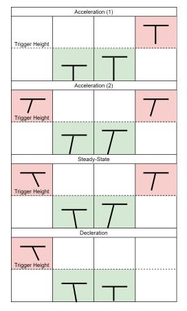
**Figure 6.4:** Diagram showing what the different states will look like. The green blocks indicate when the pneumatic cylinder should expand and the red blocks indicate when the pneumatic cylinder should contract.
