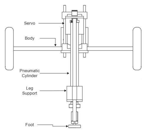
Figure 4.2: A sketch of the final robot design.
