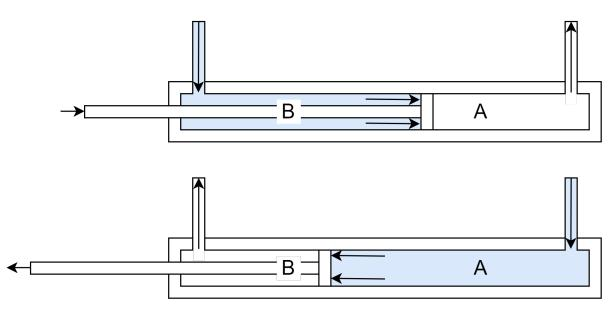
**Figure 2.5:** Pneumatic actuation explained visually, 2 chambers (A and B) are filled with air or drained of air to enable the shaft to move.
