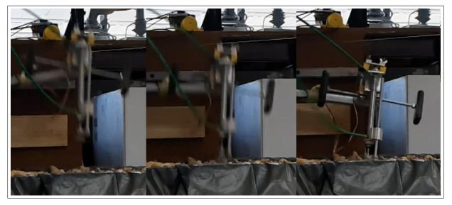
**Figure 6.8:** Screenshots of the robot showing the pneumatic expansion before the foot touches the ground.
