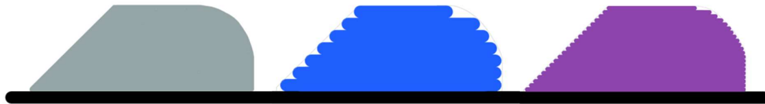
(a) Digital 3D Model (b) 0.3 mm Printed Layer Height (c) 0.1 mm Printed Layer Height
