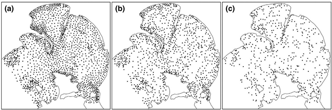
FIGURE 4 The different quantities of sounding points used during this study to conduct the three interpolation comparison tests. (a) Test 1 was conducted using the entire sounding data set, which consisted of 1,653 points. (b) Test 2 consisted of 1,091 points. (c) Test 3 consisted of 546 points
