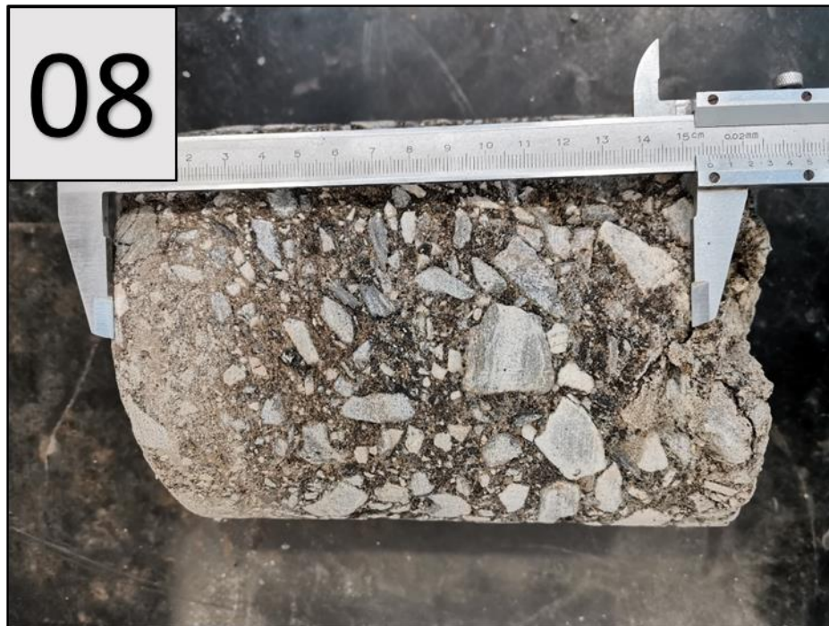
Figure 43 Irregular stone distribution in Kansanshi Specimen.
