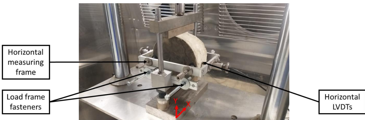
Figure 39 Positioning of the Specimen fasteners as well as the LVDTs and LVDT frame.
