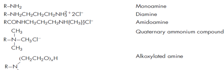
Figure 4 Chemical structures of mixtures available to create cationic emulsions provided by Redelius and Walter (2005).
