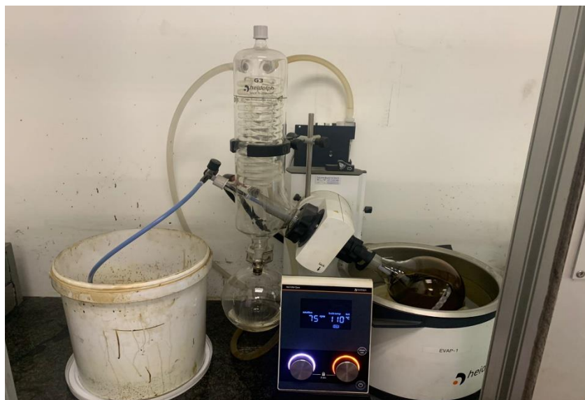
Figure 37 Rotary Evaporator used for binder extraction.
