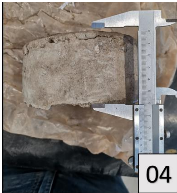
Figure 46 Layer separation observed in Specimen 4 from Kalumbila mine.
