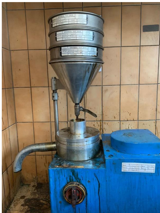
Figure 34 Centrifuge used for binder extraction.
