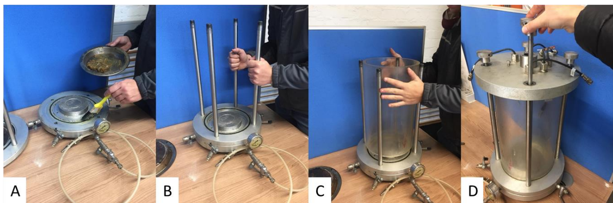
Figure 23 Triaxial loading frame construction.
