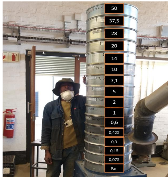
Figure 85 Grading sieves used in accordance with SANS 3310-1,2 stand-
