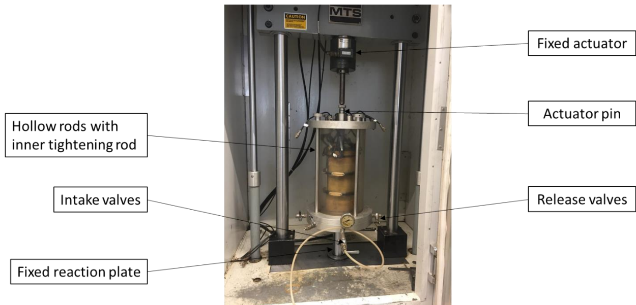
Figure 28 Complete setup of the dynamic triaxial machine.
