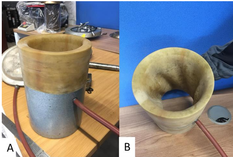
Figure 24 Side (a) and top (b) view of the rubber membrane with positioning ring.
