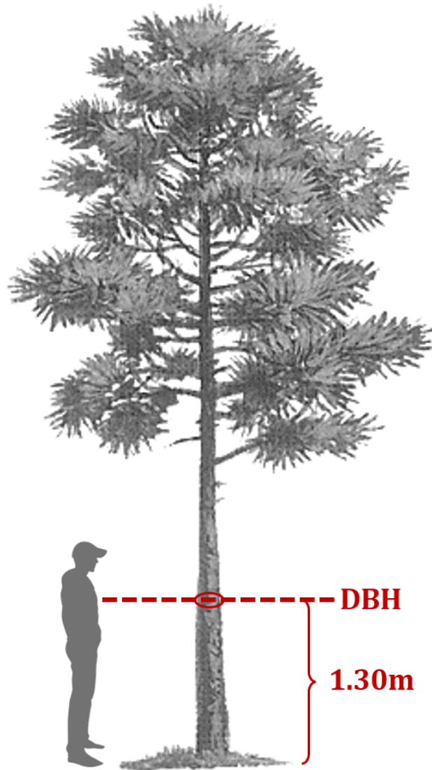
Figure 2.4: Tree characteristics and depiction of DBH height relative to an average person.
