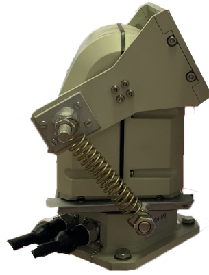
Figure 3.26: Spring used to create counter-torque.
