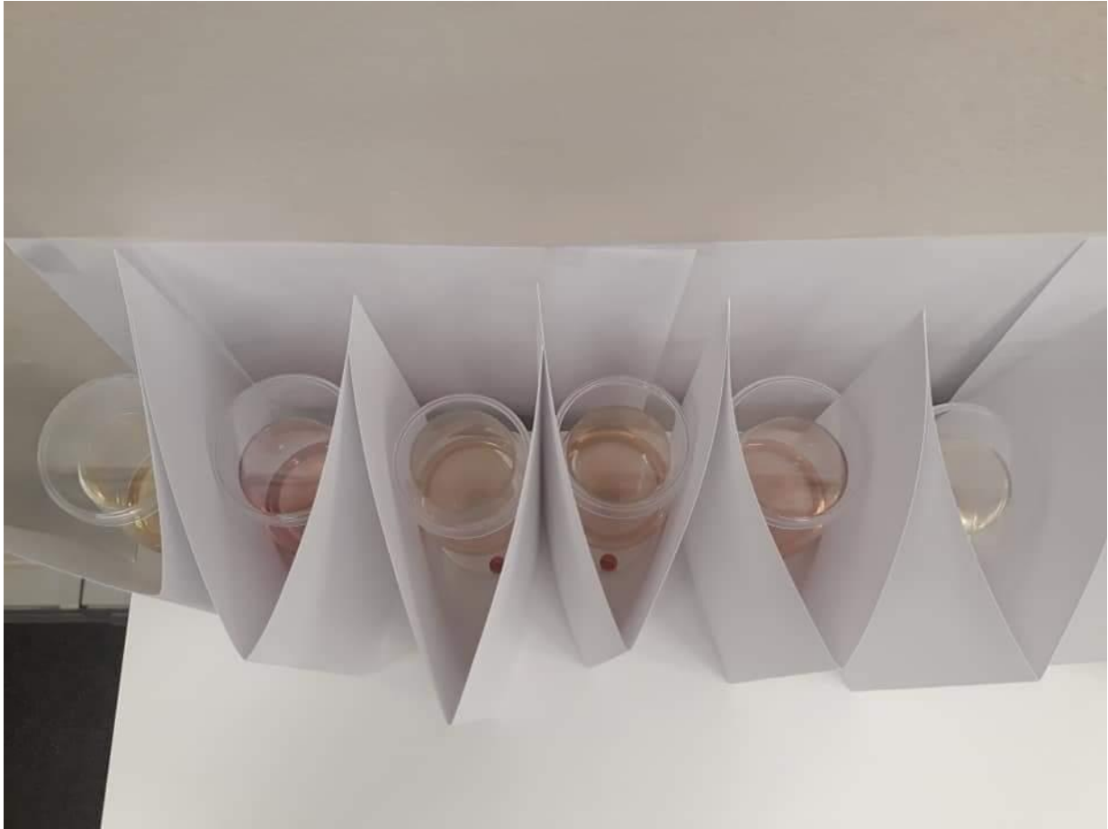
Fig. 5.2: Example of sample preparation for distinguishing between oxidised and pinked wines as wine faults. The control, oxidised and pink wines were covered with white paper so that the panelist could not see the colour of the wine. The samples were evaluated in individual tasting booths and only one sample could be uncovered at a time.
