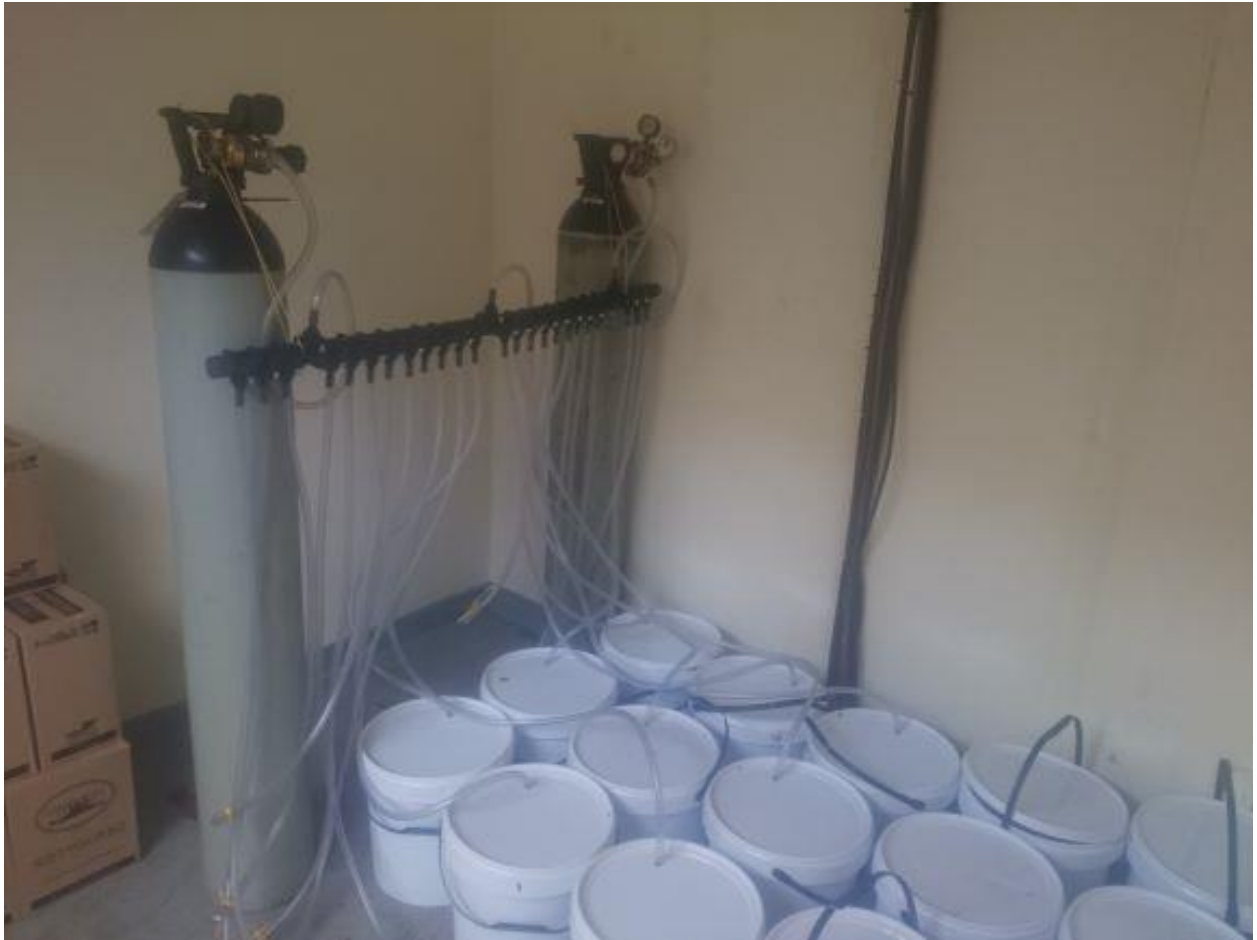
Fig. 3.1: Custom made manifold to keep macerated grape under constant CO 2 blanket for 3, 6, and 12 hours.
