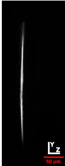
Figure 4.7: Image of the light sheet at the focal plane generated by the SLM.
