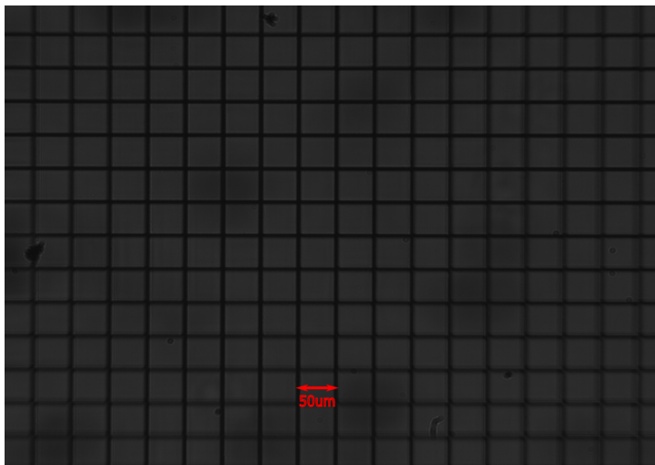
Figure 3.7: Image of the 50 \mu\text{m} grid obtained from the imaging system.
