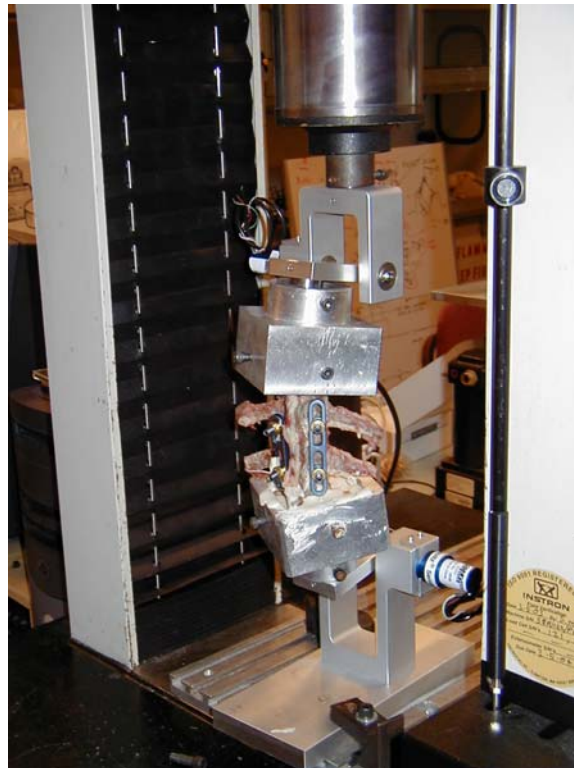
Figure 35, Cadaveric Sheep Spine in Test Stand on UTM
