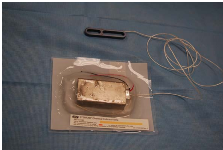
Figure 7, Instrumented Spinal Plate and Transponder
