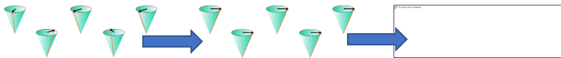
Figure 3-5 From longitudinal magnetization to transversal magnetization. The radio frequency effect on the nuclei (from Lindquist & Wager, 2013).
