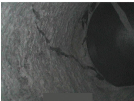
(12f) Extensive web cracking in multiple hollow-core unit ends at 2.5%
