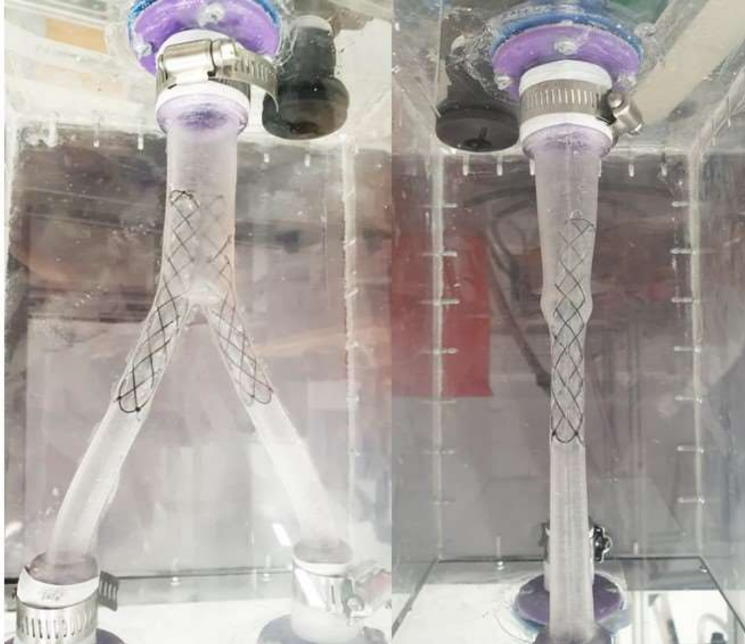
Figure 6.4: Full assembly of KS stented aorto-iliac bifurcation (left) coronal plane, (right) sagittal plane
