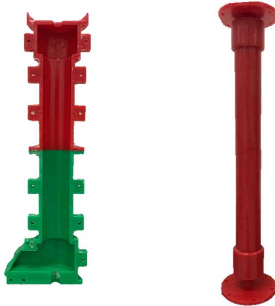
Figure 5.3: Female (left) and male (right) mould for phantom artery casting; due to the limitation of the 3D printer height, the moulds were printed in two pieces.
