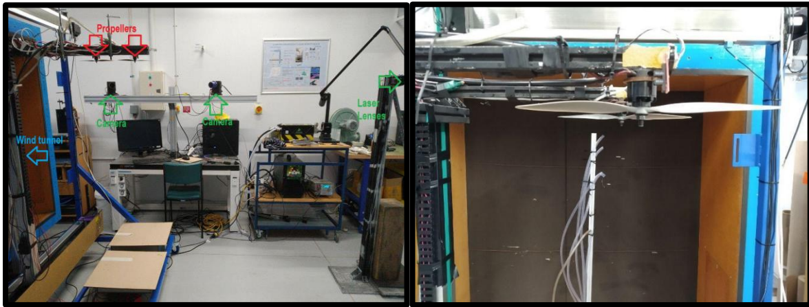
Figure 4.27 Wind tunnel setup. Two rotors (red arrows) in streamwise configuration. Labelled items are: rotors (red arrows), SPIV cameras and laser lens head (green arrows) and wind tunnel (blue arrow, pointing opposite to the direction of flow).
