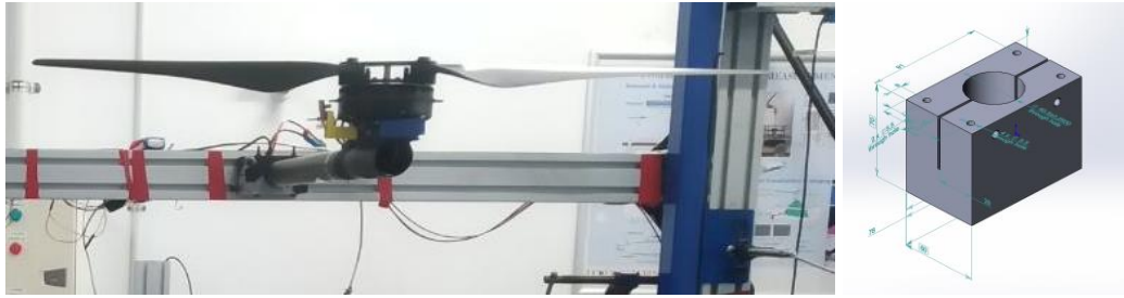
Figure 3.4 The mounting of the DJI E7000 system (left) to the aluminium slotted beam; the connector to attach the carbon fibre tube to the slotted beam (right).
