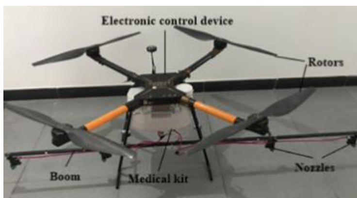
Figure 1.16 Multicopter with four 383 mm-radius rotors and four attached spraying nozzles (Wen et al., 2019)
