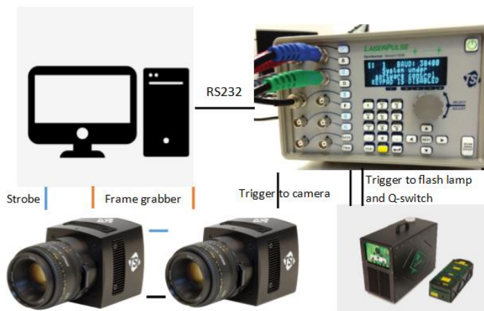
Figure 2.2 Key components and their connection in the SPIV system.
