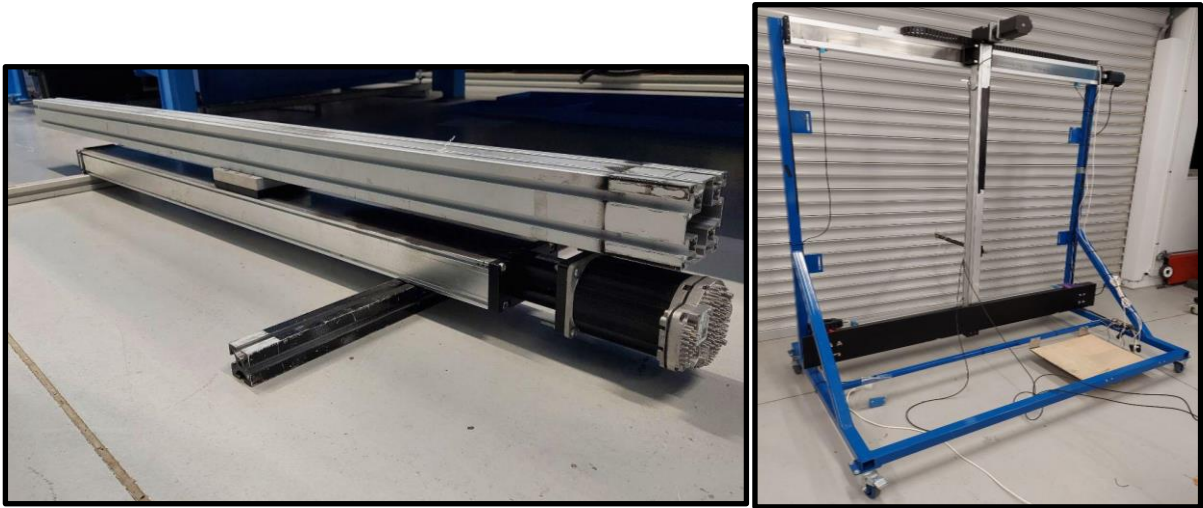
Figure 2.20 Traverse used in experiments; left: one-dimensional traverse, right: two-dimensional traverse.
