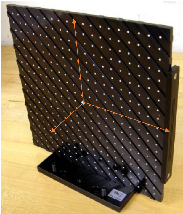
Figure 2.14 Four plane target with predefined dot grid used for SPIV calibration.
