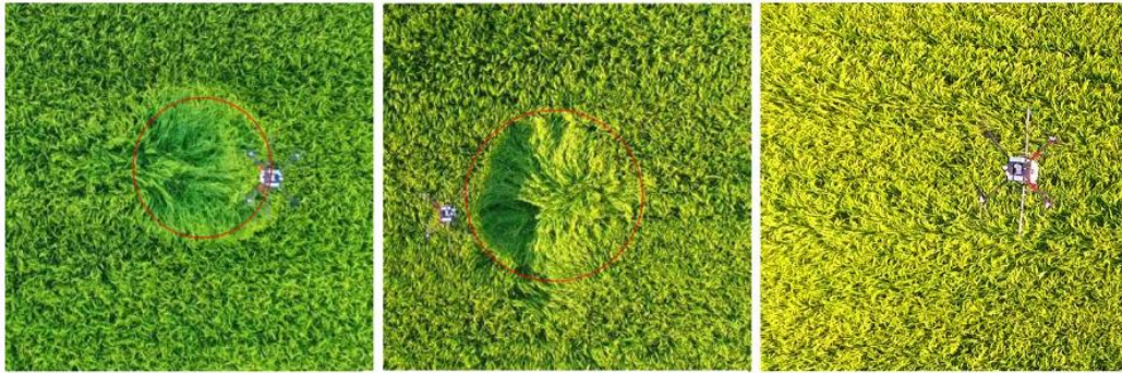
Figure 1.15 Rice plant response to the wake of a flying multicopter: (left) height 1.2 m, flight speed 1.4 m/s; (centre) height 2.4 m, flight speed 2.4 m/s; (right) height 5.1m, flight speed 3.4 m/s (Guo et al., 2021)
