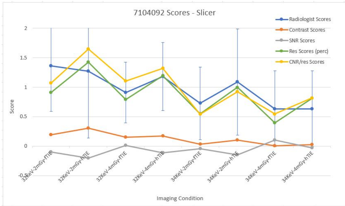
Figure A.19: Plot of subjective radiologist scores (in blue) for each imaging condition for sample 7104092 (shown in Table 3.3), with error bars of \pm one standard deviation (shown in Table A.2). The subjective radiologist score is compared to various scaled quantitative scores measured using 3D Slicer including; CNR/res (yellow), contrast (red), SNR (grey) and spatial resolution (green) for sample 7104092.
