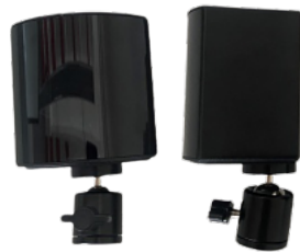
Figure 3.19: Two SteamVR 2.0 Base Stations [59].
