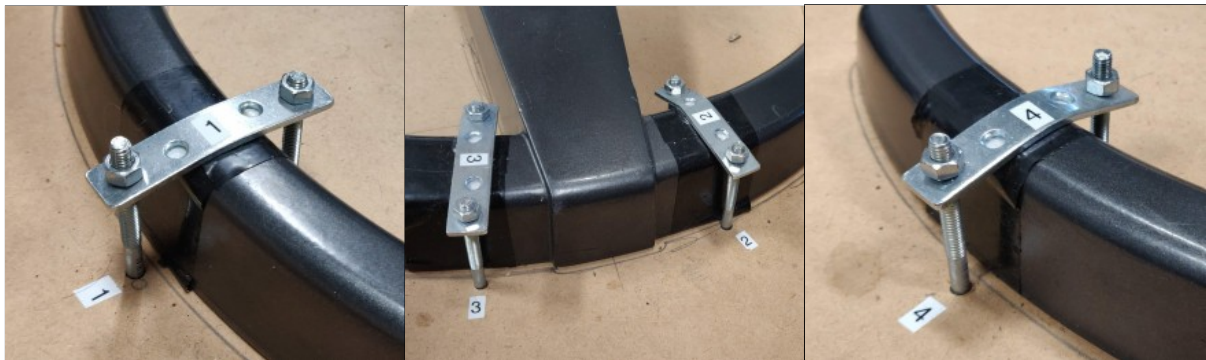
Figure 3.3: The fastening of the Swopper stool to the MDF base.
