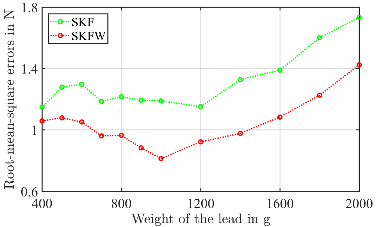
Fig. 5.8. The RMSE of the external force estimation based on the SKF and the SKFW from 400 g to 2000 g.
