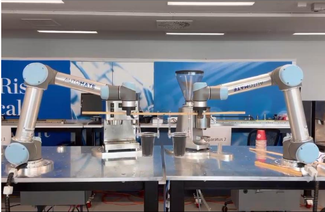
(c) Two UR5 move up at constant speed as the TCP does.
