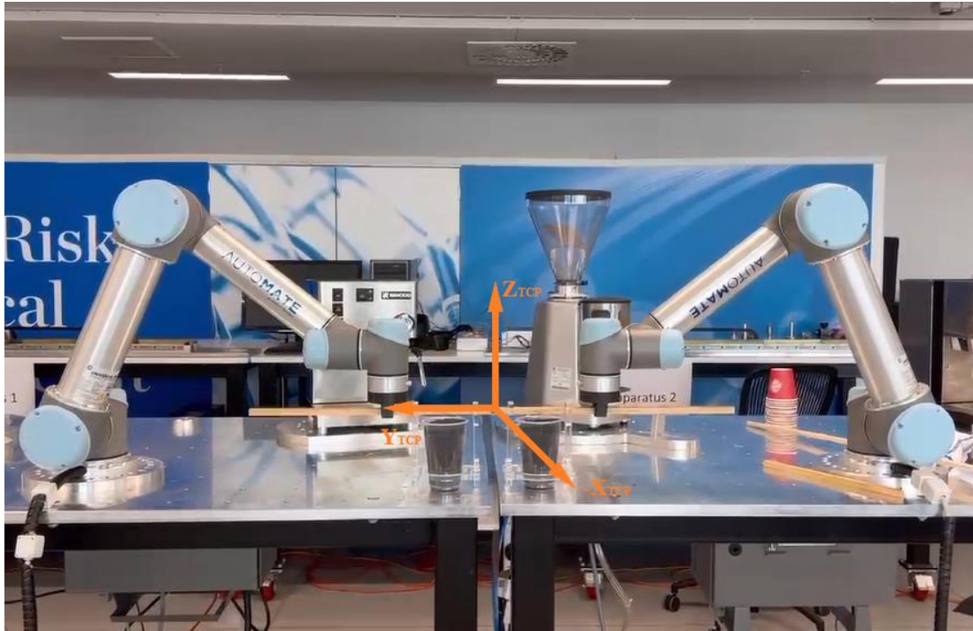
(a) Initial pose. Two UR5 are coupled by a batten. The TCP is located in the middle of the batten and goes up at constant velocity of 0.06\text{m/s} . Initially the cups are not engaged.
