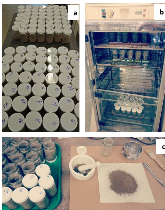
Plate 3.1 Glass jars with treated soils (a), incubator (b) and soil grinding and sieving after drying at the end of the incubation (c).
