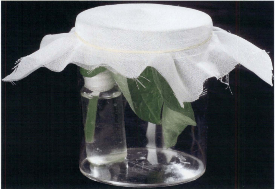
Figure 2.1 An example of the experimental setup for PTM bioassay with excised leaves
