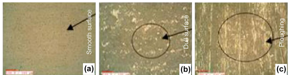
Fig. 48 Micrographs for aluminium alloy 5005 specimens a un-peened surface b WJP with single pass and c WJP with double passes [167]
