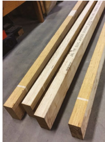
(b) Laminated veneer lumber (LVL11)
