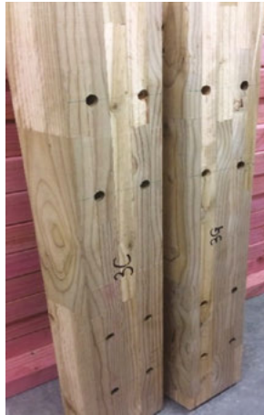
(a) Glued laminated timber (PL8)
