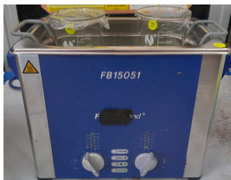
Fig. 6. Ultrasonication treatment process on Al 2 O 3 /POE nanolubricants.
