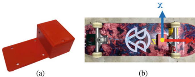
Fig. 2 The sk8pro device attached at bottom front of the board a the 3D printed sk8pro device b attachment of the sk8pro to the skateboard
