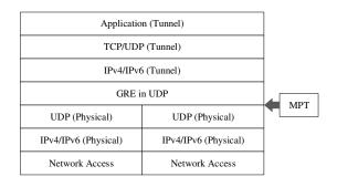
Figure 1. Layered architecture of the MPT-GRE.
