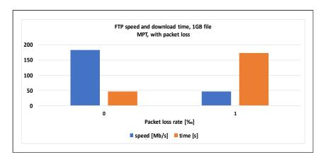
Figure 8. The effect of the packet loss on the FTP throughput and download time.
