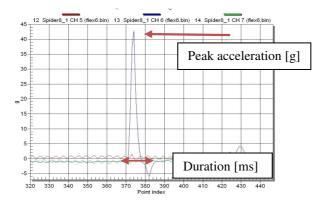
Figure 5. Registered shock during a drop on a packaged product (source: Authors)
