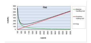
Figure 3: Total cost in function of packaging unit quantity
