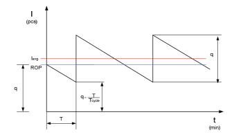
Figure 2. Inventory diagram of single production lines
