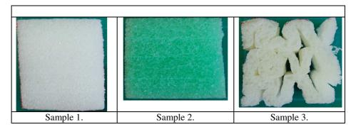
*Figure 4. 3 type of foam, applied as a cushion material (source: own photo)*
