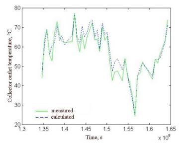
Figure 5: Collector outlet temperature values after parameter identification
