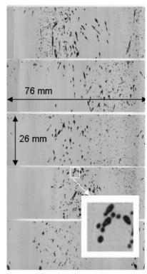
Fig. 12 Water sensitive paper sample used at investigation of a TX ConeJet VK 26 type nozzle at work.
