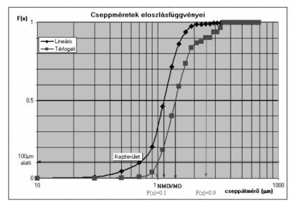
Fig. 14 Droplet structure by a rotation nozzle of type Micron X1 at rpm  $n=1410 \ 1/min$ .
