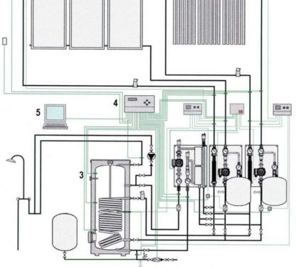
1. flat plate collectors; 2. vacuum tube collectors; 3. hot water tank; 4. HC-23 microprocessor based data acquisition system; 5. computer Figure 1: The sketch of the solar thermal system
