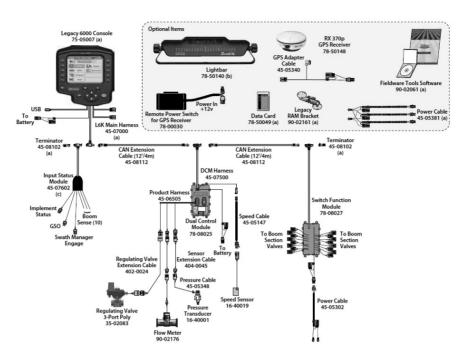
Fig. 3 Schematic overview of FieldPilot on a plant protection sprayer.
