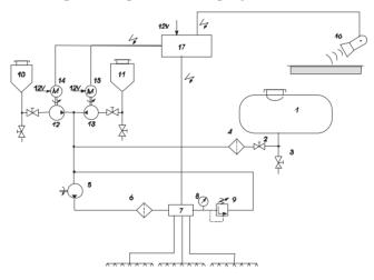
Fig. 6 On-line pesticide feeding
