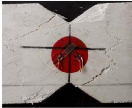
Figure 4.11: Crack growth in an Iosipescu test sample with fibre orientation (a) \pm 15^\circ and (b) \pm 75^\circ .
