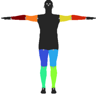
Figure 3. The used norm pose depicted with the fixed keypoints from the COCO dataset.
