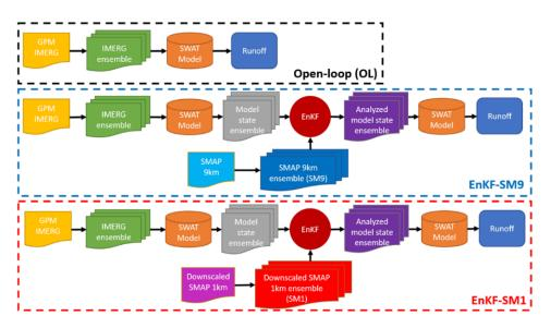
**Figure 2.** Flow chart of this study. EnKF-SM9 and EnKF-SM1 stand for streamflow simulations using the SWAT model with the state variable of SM9 and EnKF technique, and streamflow simulations using the SWAT model with the state variable of downscaled SM1 and EnKF technique, respectively.
