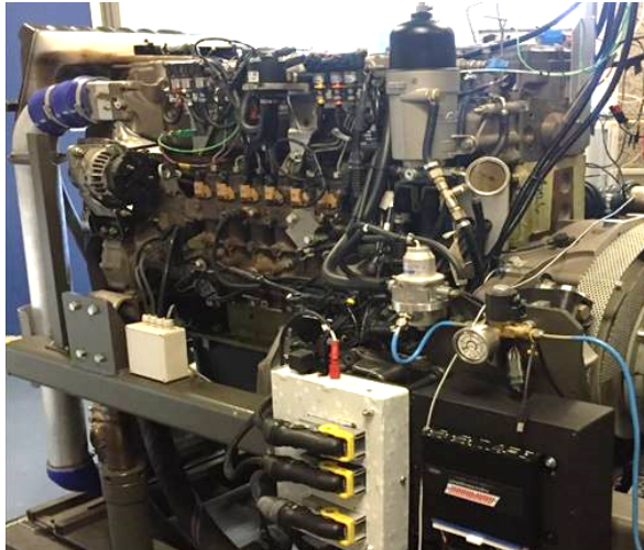
Figure 11 DAF PR 6-cylinder engine in test cell, intake side.
