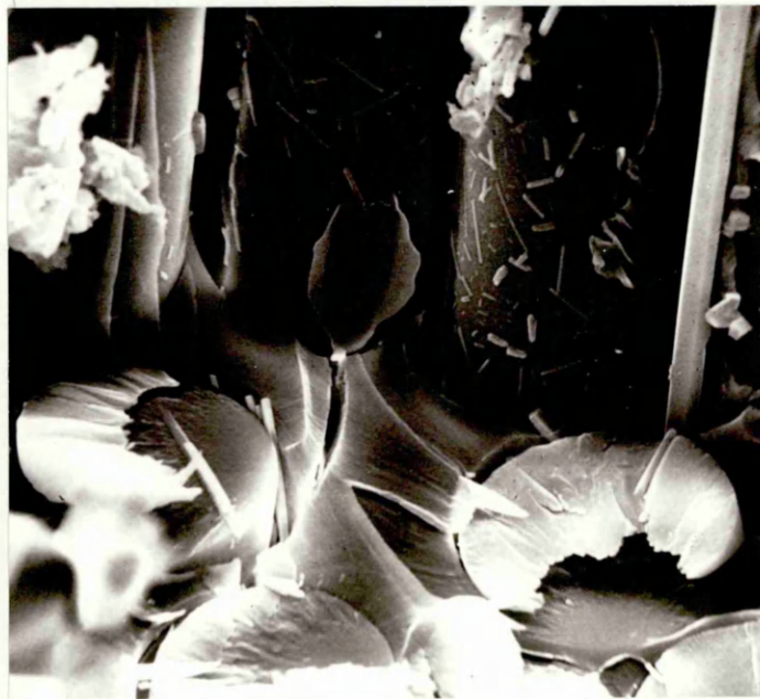
Figure 3.28 Micrograph showing glass segments produced when bifurcation of the fracture crack occurs in the glass fibre.
