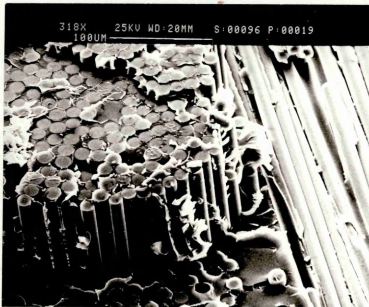
Figure 3.30 Mode II fracture surface showing steps.
