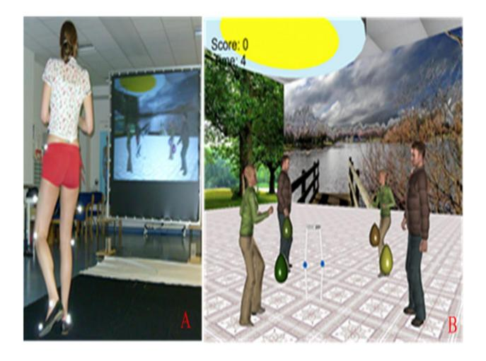
*Figure 3*: A clinical engineer trainee using the SVRS to perform the third test (clearing obstacles exercise). A: during the actual test and B: a screenshot of the VR environment.
