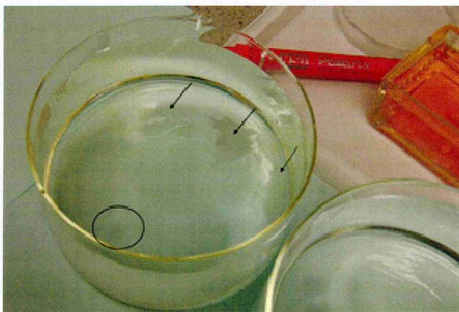
Figure 5.2: (Top) Process flow for transferring as grown graphene from the metal catalyst onto another substrate – in this case \text{SiO}_2 support for further processing and analysis. (Bottom) Graphene film floats on the water surface after the previous step of removing the metal substrate (indicated by the circle highlight). Note the arrows referred to water trapped underneath the glassware and reflections from surroundings.
