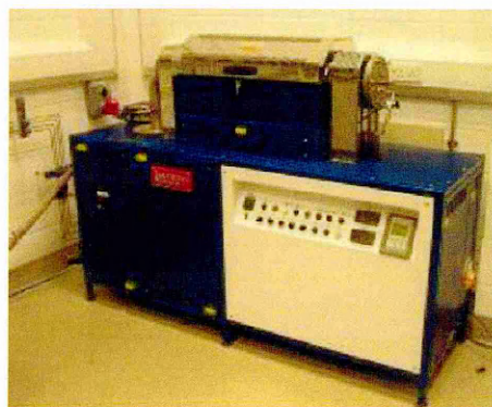
Figure 3.2: (Top) Cross-sectional diagram of a T-CVD furnace used in this study [7] and (bottom) photograph of the equipment. The metal plates in the schematic are placed near the both ends of quartz tube to reduce a distribution of heat at the middle of the quartz tube and to avoid the excess heating up of flange which possibly results in degreations of o-rings in the franges.
