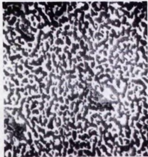
No. 26 R_s = 290 \Omega/\square , 6.2 \times 10^{15} Ions/cm 2
