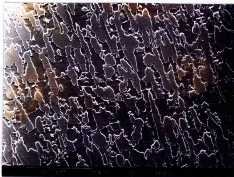
Figure 6-70 An SEM micrograph taken from the GRY steel sample exposed in 10%wt HCl for 2 hours.
