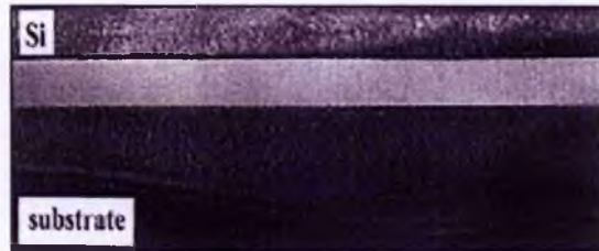
Figure 4: Shows a Simox XTEM cross section with the silicon over layer on top and BOX (buried oxide layer) in the middle and substrate underneath [24].
