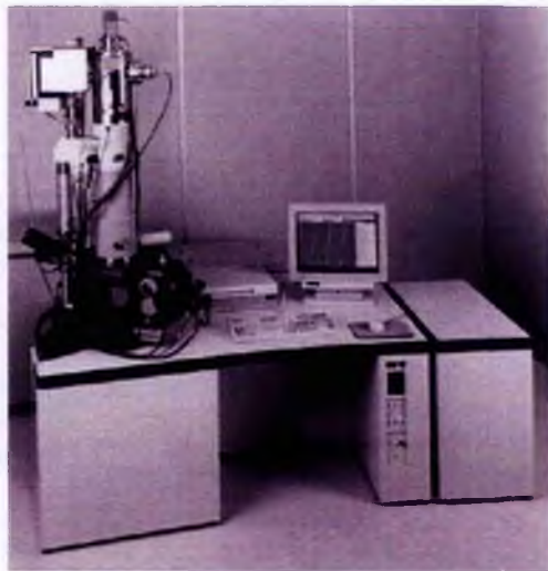
Figure 30 shows the e-beam lithography system used [104].
