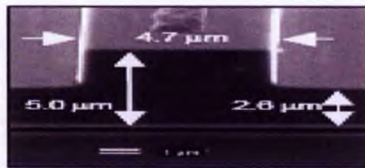
Figure 27 shows a SEM of the rib waveguide used in Taaed's work [101].
