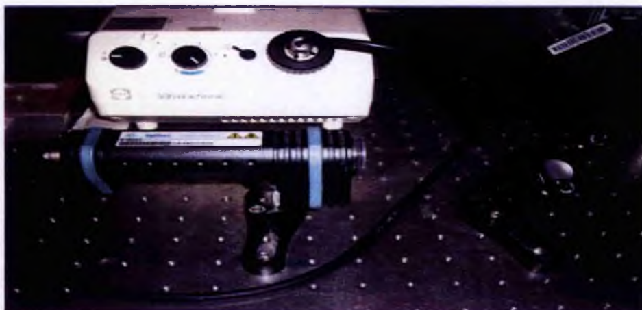
Figure 70 the variable lamp and detector and flip-up mirror in the foreground. The flip-up mirror (figure 70) to the left of the left hand lens and xyz micrometers are to be carefully elevated (thus avoiding damage to its internal spring) and the light from the variable incandescent lamp (set to about 3) taken via the optic cable to the
