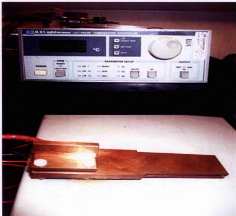
Figure 103 temperature response experiment (a) Peltier temperature controller, (b) Copper Carrier.
