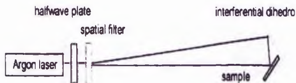
Figure 21 schematic of holographic setup [94].
