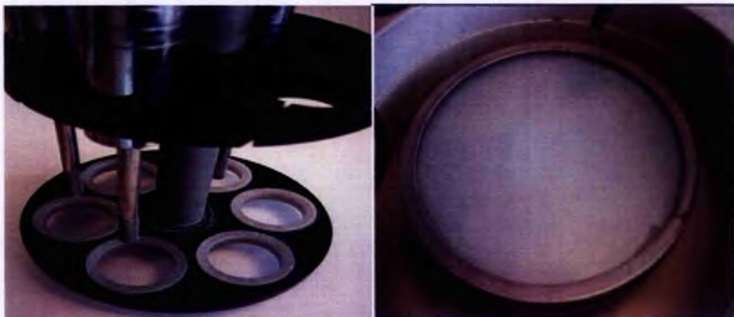
Figure 68 Outer Metal Retaining Ring Glass platen, Sample Holder and Retaining Clamp.
