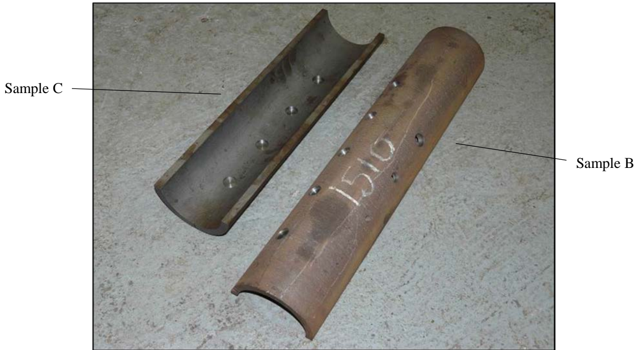
Figure 6.3 - Samples B and C after preparation for magnetic inspection showing internal and external machined defects.
