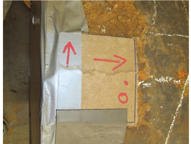
Figure 8.4 - Detail of the end caps that covered each end of the pipes and the caps covering each v-notch: (a) Pipe 2 with its end caps in place and (b) A cap covering a v-notch on Pipe 2 with the positive measurements directions and measurement origin drawn on.
