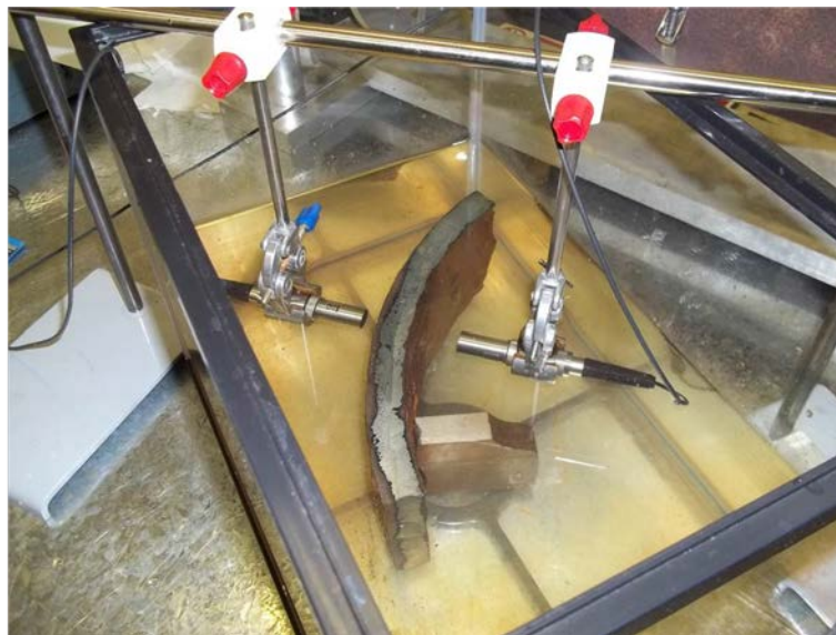
Figure 5.13 - Ultrasonic pulse-echo testing carried out in immersion on a section of graphitised cast iron.
