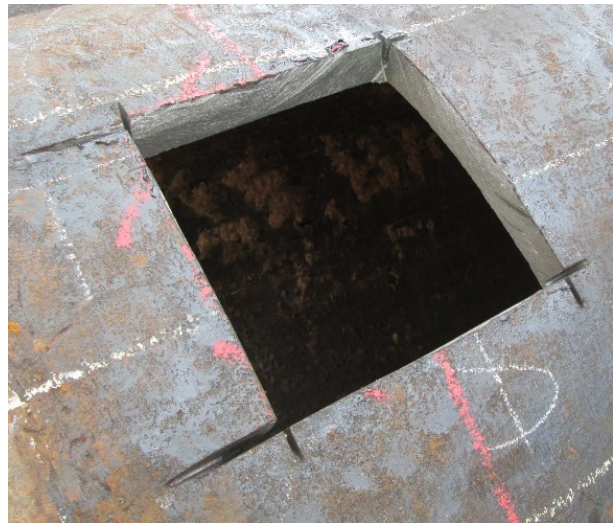
Figure 7.21 - Additional reference markers cut into Specimen Three: (a) the complete pipe section with reference markers, (b) a close-up of a diamond marker and (c) a close-up of a square marker.
