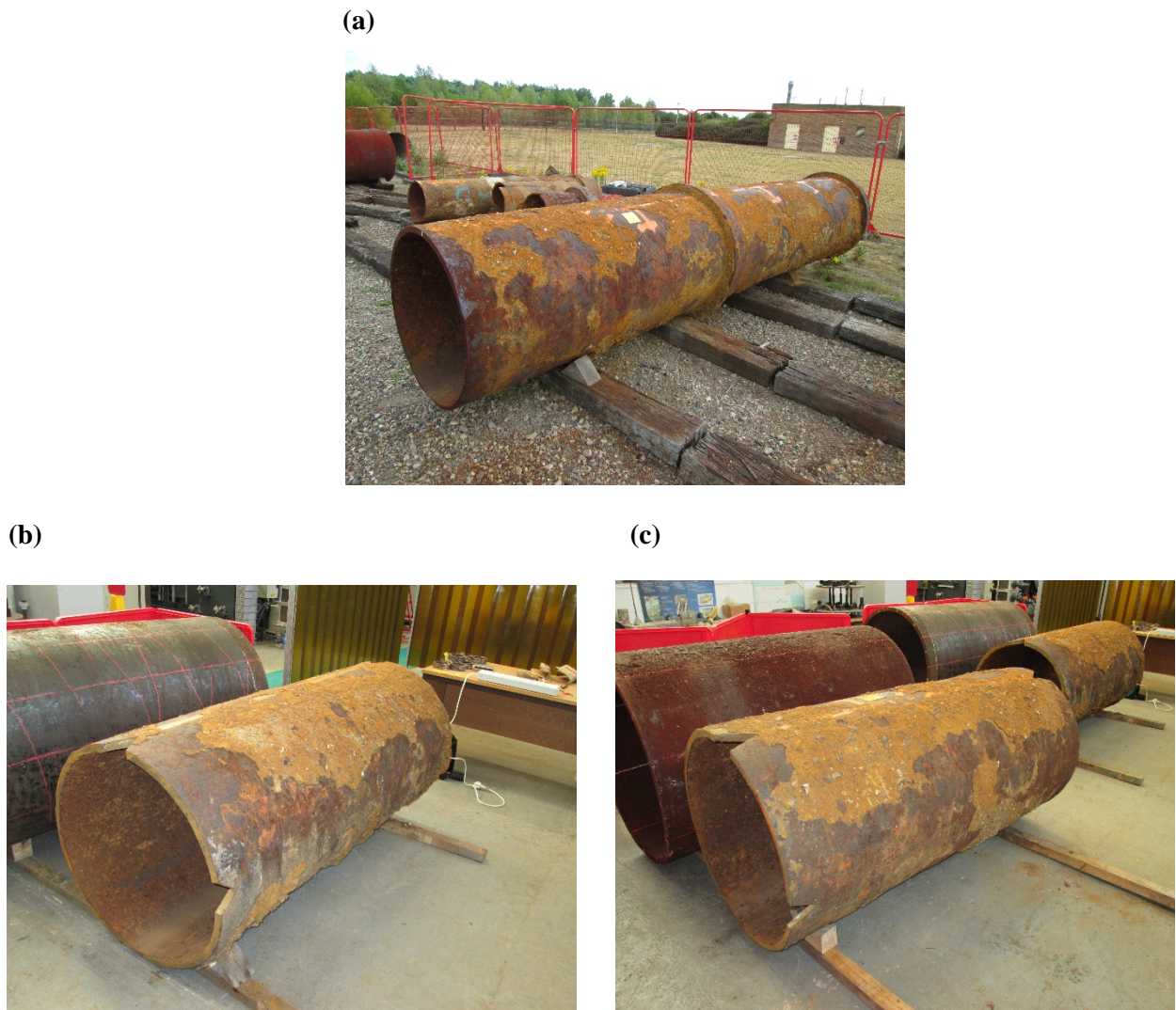
Figure 8.2 - Jointed pipe cut-out before and after it was cut into smaller sections: (a) complete pipe cut out, (b) Pipe 1 and (c) Pipe 2
