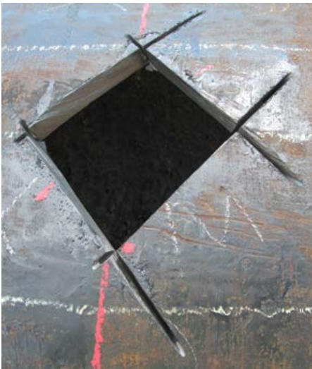
Figure 7.21 - Additional reference markers cut into Specimen Three: (a) the complete pipe section with reference markers, (b) a close-up of a diamond marker and (c) a close-up of a square marker.
