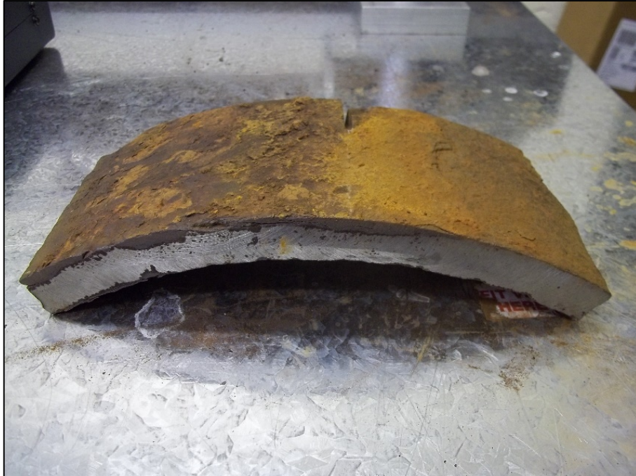
Figure 6.2 - Sample A, which was used for feasibility testing the magnetic force testing principle.
