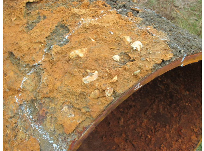
Figure 8.3 - Different types of surface encrustation found across the surface of both pipes: (a) a very hard pointed encrustation formation and (b) a softer encrustation formation including stones from the surrounding soil.
