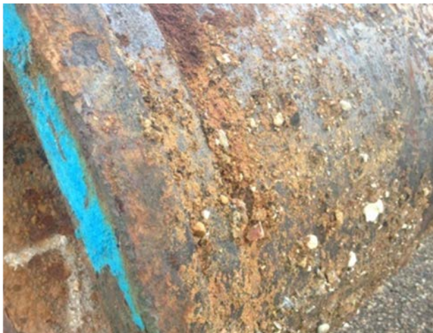
Figure 4. 3 - Barriers to NDE on cast iron trunk main: (a) surface encrustation and (b) variable geometry.
