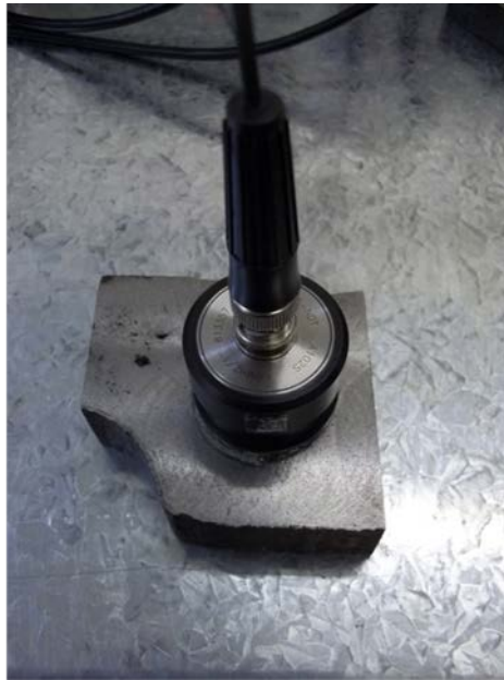
Figure 5.12 - Contact ultrasonic transducer being used to measure the velocity of sound in a machined section of cast iron
