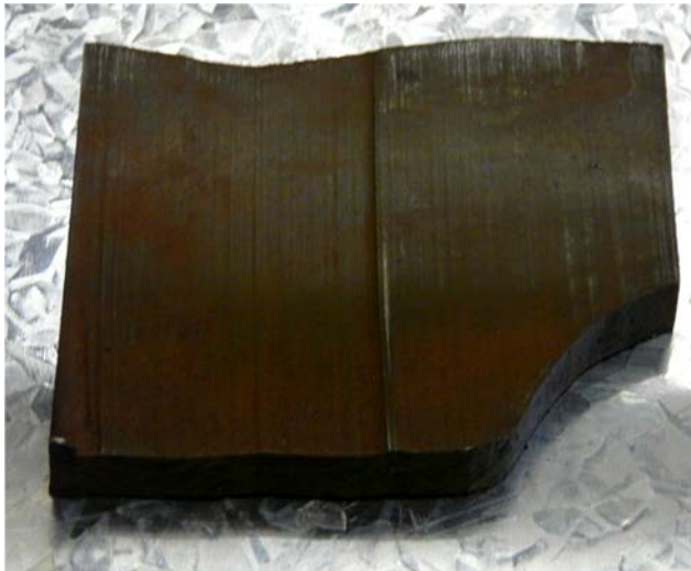
Figure 5.9 - Samples taken from cast iron flange: (a) water-jet cutting finish and (b) as machined surface
