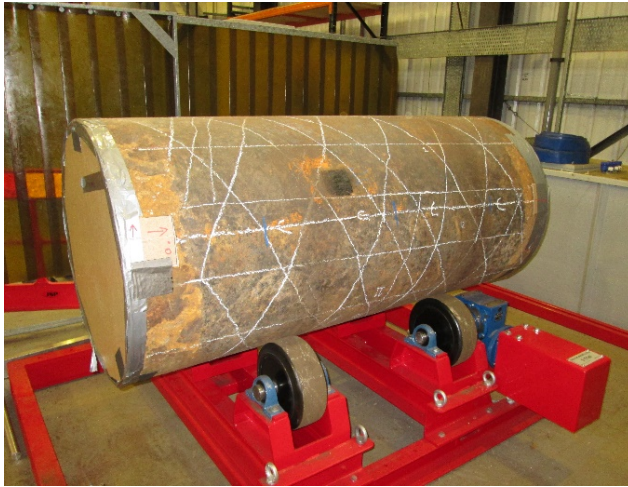
Figure 8.4 - Detail of the end caps that covered each end of the pipes and the caps covering each v-notch: (a) Pipe 2 with its end caps in place and (b) A cap covering a v-notch on Pipe 2 with the positive measurements directions and measurement origin drawn on.
