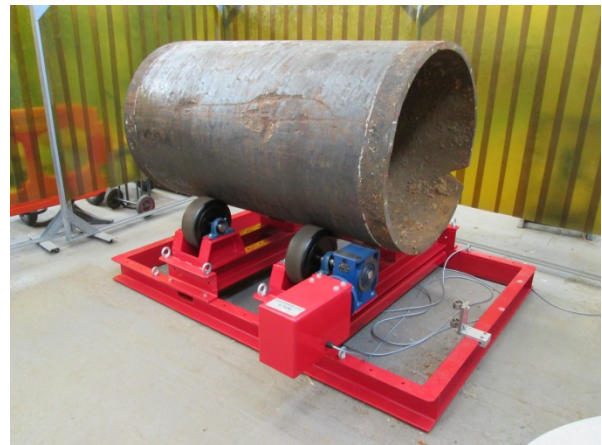
Figure 7.4 - Equipment used to conduct the pipe scanning: (a) the Artec Eva structured white light scanner (Artec, 2016) and (b) the specialised pipe rotator used to manipulate the sections of trunk main loaded with a section of 42” main.
