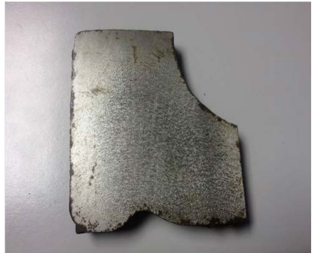
Figure 5.9 - Samples taken from cast iron flange: (a) water-jet cutting finish and (b) as machined surface
