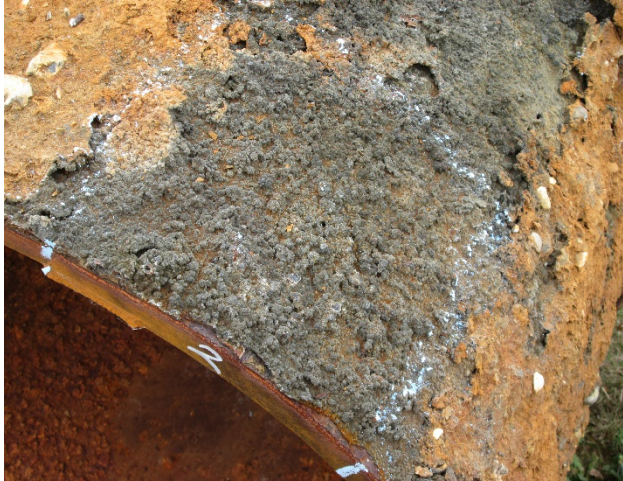
Figure 8.3 - Different types of surface encrustation found across the surface of both pipes: (a) a very hard pointed encrustation formation and (b) a softer encrustation formation including stones from the surrounding soil.
