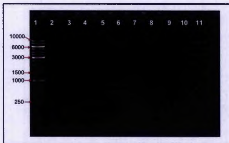
Figure 5.3: Agarose-gel electrophoresis of pDNA binding to CNT. Lane 1 – 1 Kb Ladder; Lane 2 and 3 – Poly(Lys:Phe) or PL-PEG-NH 2 respectively, conjugated with DNA wrapped around oxidised DWNTs (Lane 2 – Poly(Lys:Phe)-pDNA-oxDWNT; Lane 3 – PL-PEG-NH 2 -pDNA-oxDWNT); Lane 4 - pristine DWNT wrapped with Poly(Lys:Phe) (Lane 4 - DWNT-Poly(Lys:Phe)-pDNA); Lane 5 and 6 - oxidised DWNT wrapped with Poly(Lys:Phe) or PL-PEG-NH 2 , respectively and conjugated with pDNA (Lane 5 – oxDWNT-Poly(Lys:Phe)-pDNA; Lane 6 – oxDWNT-PL-PEG-NH 2 -pDNA); Lane 7 and 8 – similar to 5 and 6 but using single-walled CNTs (Lane 7 – oxSWNT-Poly(Lys:Phe)-pDNA; Lane 8 – oxSWNT-PL-PEG-NH 2 -pDNA); Lane 9 and 10 – controls Poly(Lys:Phe)-pDNA and PL-PEG-NH 2 -pDNA, respectively; Lane 10 – pDNA control.
