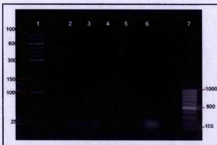
Figure 5.4: Agarose-gel electrophoresis of siRNA binding to CNT. Lane 1 – 1 Kb Ladder; Lane 2 – PL-PEG-NH 2 conjugated with siRNA wrapped around oxidised DWNTs (Lane 2 – PL-PEG-NH 2 -siRNA-oxDWNT); Lane 3 - pristine DWNT wrapped with PL-PEG-NH 2 and conjugated with siRNA (Lane 3 - DWNT-PL-PEG-NH 2 -siRNA); Lane 4 – Poly(Lys:Phe) conjugated with siRNA wrapped around oxidised DWNTs (Lane 4 – Poly(Lys:Phe)-siRNA-oxDWNT); Lane 5 - pristine DWNT wrapped with Poly(Lys:Phe) and conjugated with siRNA (Lane 4 - DWNT-Poly(Lys:Phe)-siRNA); Lane 6 – siRNA control; Lane 7 – 100 bp Ladder.
