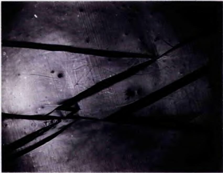
Fig. 3.9 Twin intersections and cross-twinning showing accommodation slip and kinks (x 80)
