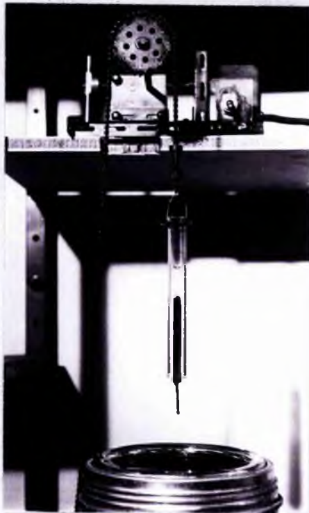
Fig. 2.4 Crystal growth equipment prior to growth of single crystal.
