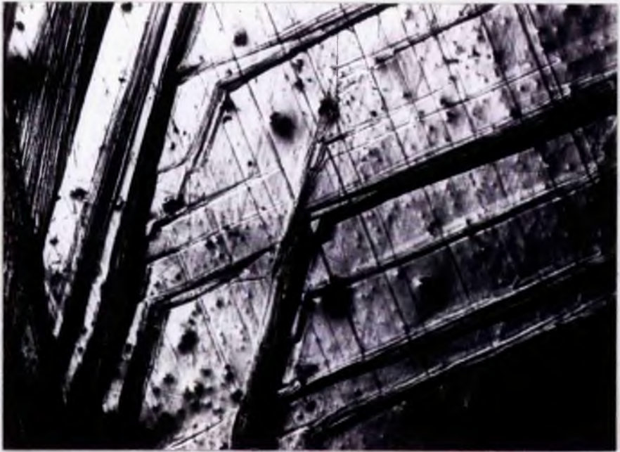
Fig. 5.5 Close-up of crystal in Fig. 5.4 showing obtuse intersections between plates of \gamma -mercury (x 80)
