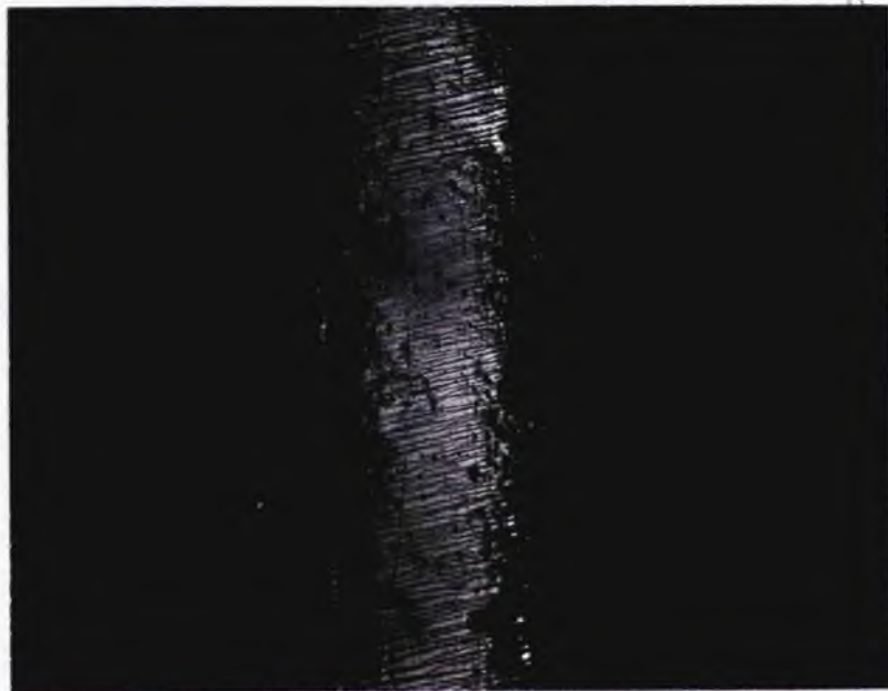
Fig. 1.2 Example of wavy slip on a cylindrical crystal
