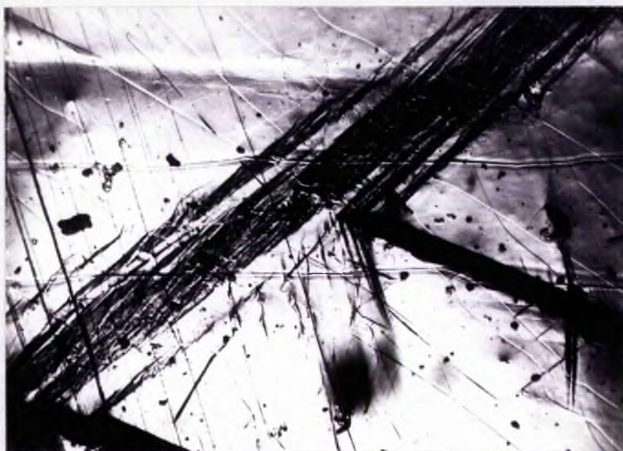
Fig. 5.3 Twin intersection showing accommodation slip (x 100)
