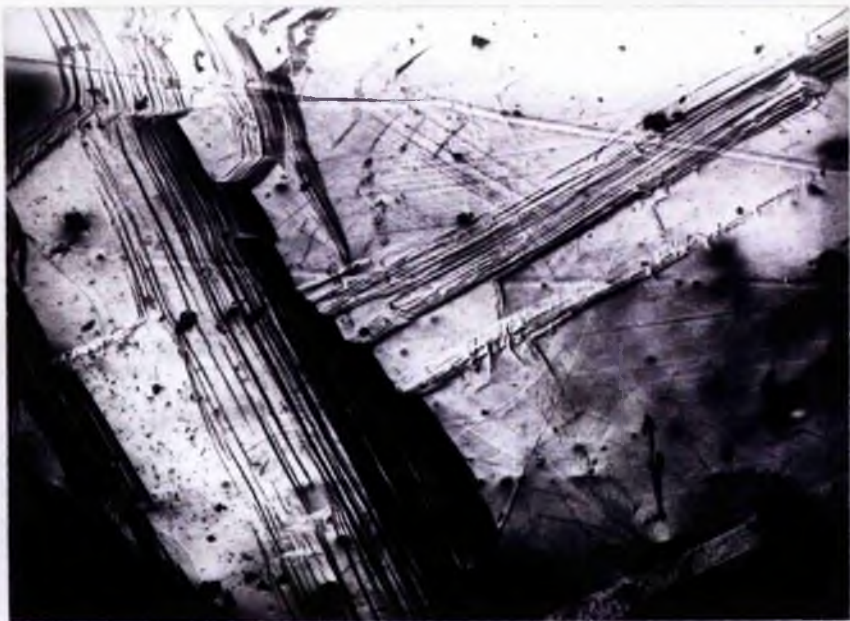
Fig. 5.8 Reduction of interface energy by occurrence of complementary modes (x 100)
