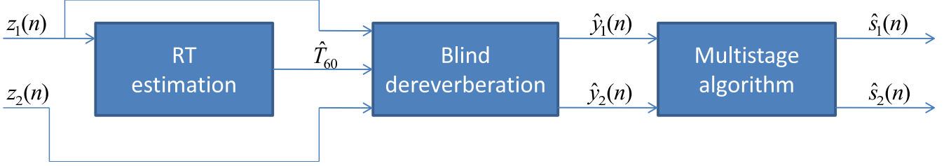
Figure 1: Block diagram showing the first scheme for the proposed joint blind dereverberation and separation algorithm. z_1(n) and z_2(n) are the available mixtures (microphone signals).
