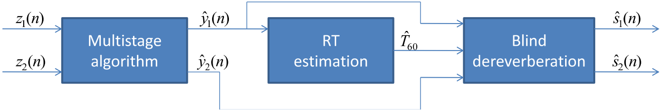
Figure 2: Block diagram showing the second scheme for the proposed joint blind dereverberation and separation algorithm. z_1(n) and z_2(n) are the available mixtures (microphone signals).
