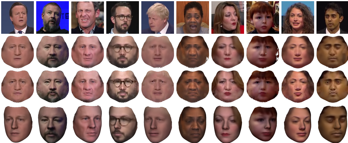
Fig. 4. (Top row): Frame from the original video. (Second row): Reconstructed face texture using our real-time method. (Third row): Ground truth face texture. (bottom row): Rendering of a novel pose.
