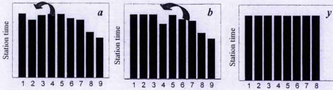
Figure 3.2. Progressive loading of workstations: solution (a) first station is packed; solution (b) first three stations are packed; solution (y) all the stations are fully packed and total number of stations equal to eight.
