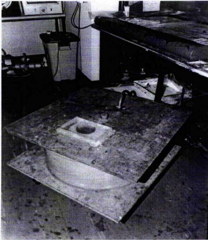
Figure 3.4.- Vacuum system for resin impregnation.
