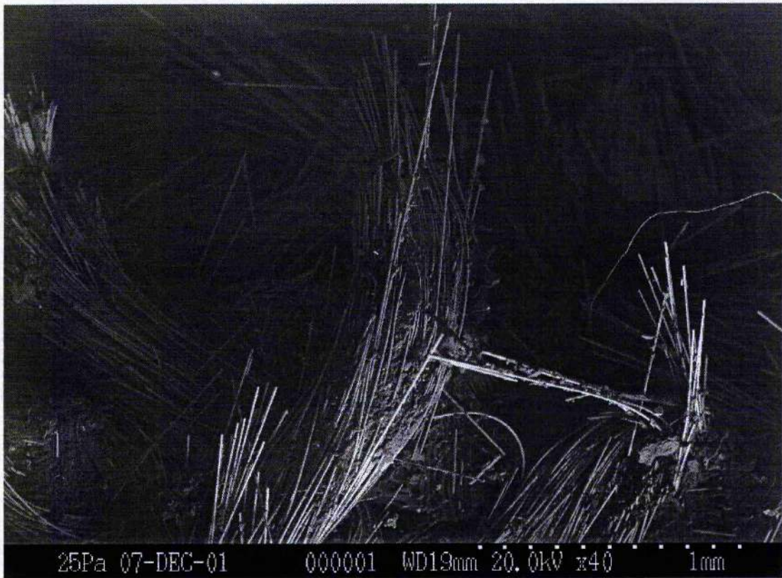
Figure 5.25.- Fractured surface of RTM sample tested in the -45^\circ direction.
