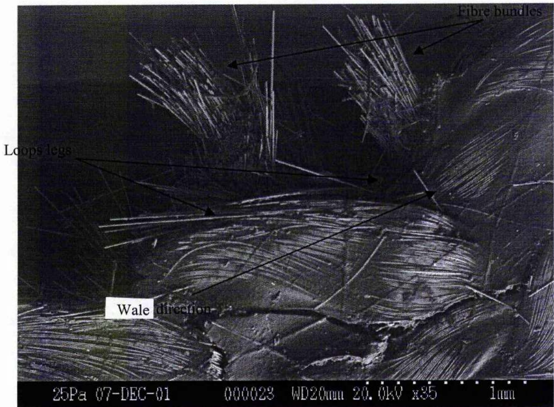
Figure 5.31.- Fractured surface of RTM sample tested in the 60° direction.
