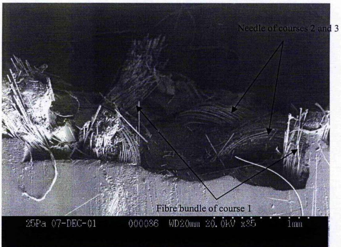
Figure 4.23.- Fractured surface of single layer sample tested in the 0^\circ (wale) direction.
