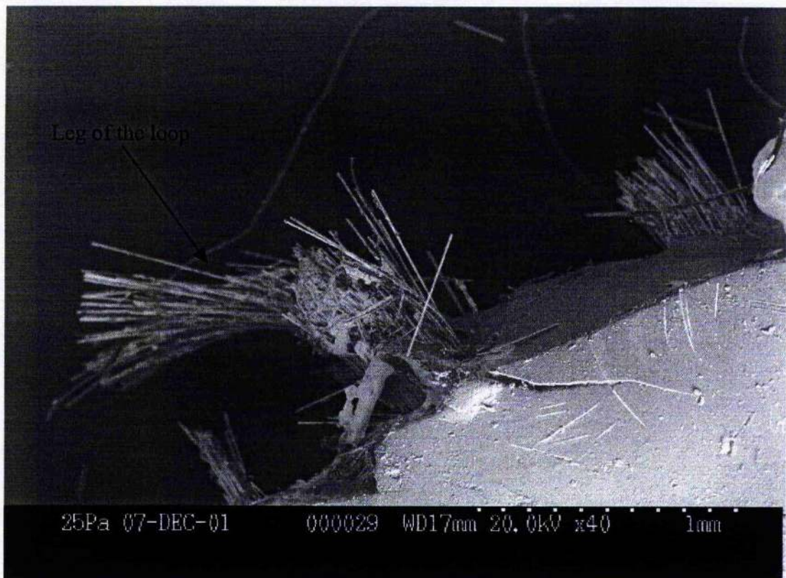
Figure 4.24.- Fractured surface of single layer sample tested in the 30° direction.
