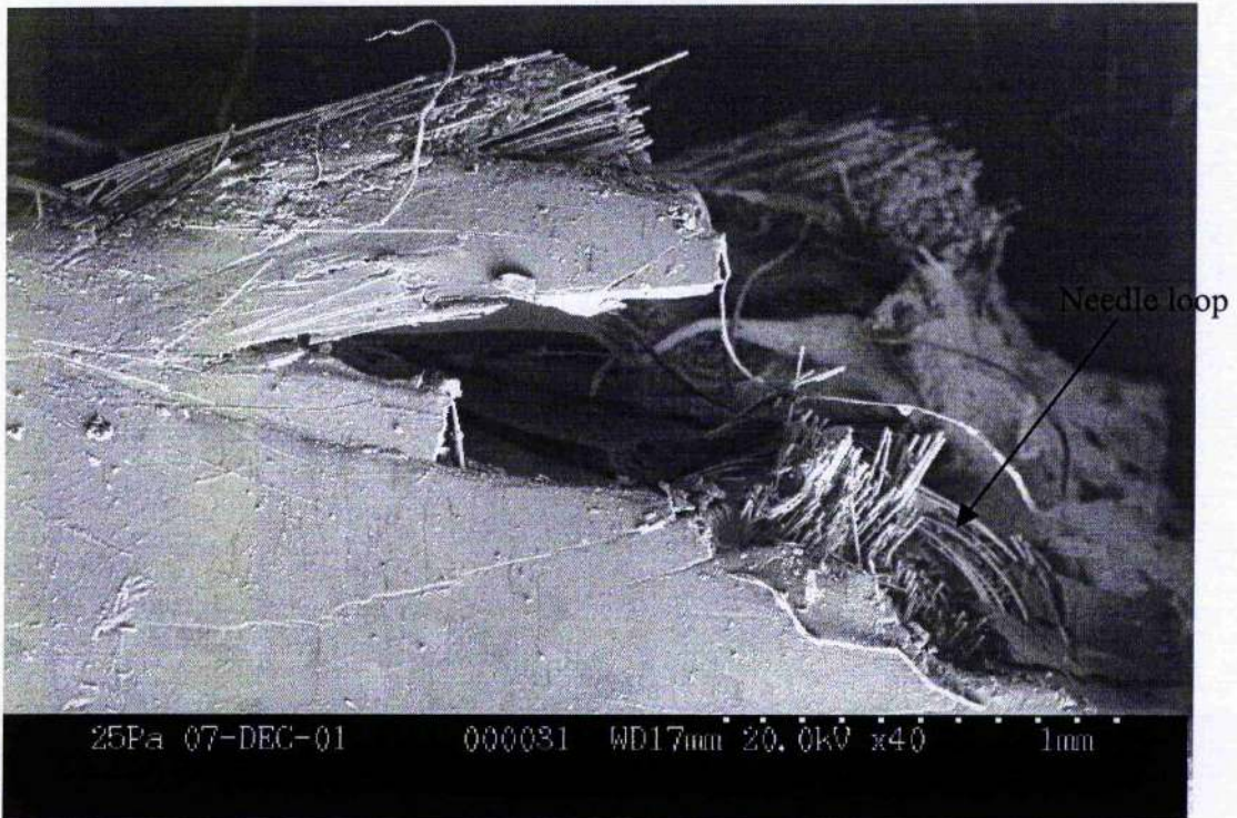
Figure 4.24.- Fractured surface of single layer sample tested in the 30° direction.
