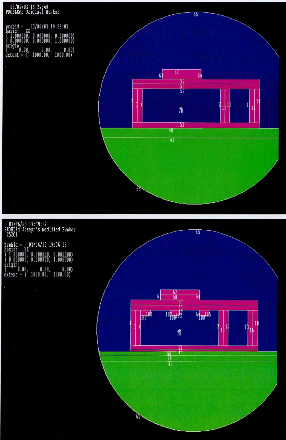
Fig. 8.5a: MCNP geometry plot of the transverse view of the original and modified bunker showing the primary and secondary shielding and the baffles in the ceiling of the treatment room in the case of the modified bunker.
