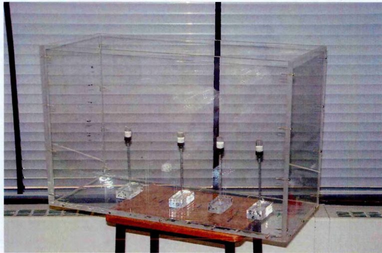
Fig. 6.8: A 25 \times 60 \times 45 \text{ cm}^3 (internal dimensions) Perspex water phantom used for the in phantom measurements. The SDDs are as shown in the erect (irradiation) position.
