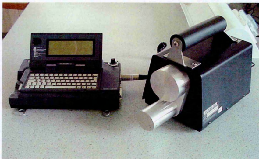
Fig. 3.3: The neutron probe (N-Probe) and Atari Portfolio palm-top computer with a LCD screen. (By kind courtesy of the Nuclear Department, HMS Sultan, Gosport, UK)
