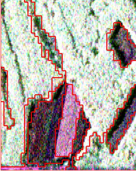
Fig. 11. Segmentation results with the KummerU criterion for the L-band ESAR data over the Oberpfaffenhofen test site ( 500 \times 400 pixels). Partition containing ten segments over a colored composition of the target vector [k]_1 - [k]_3 - [k]_2 .
