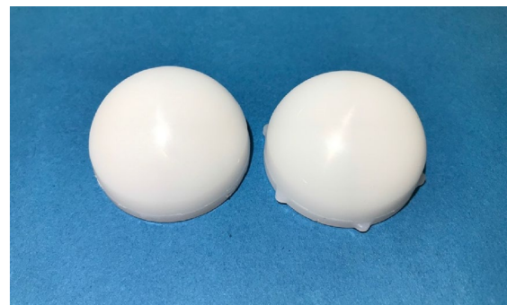
Fig. 5 3D CAD image showing the Pinnacle liner [left with the anti-rotation tabs (ARTs) removed; on right ARTs intact]
