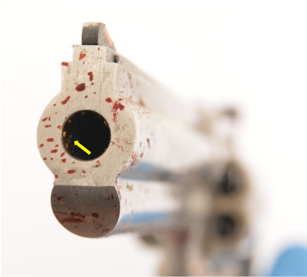
Fig. 5 GSRs at the inside of the muzzle (yellow arrow)
