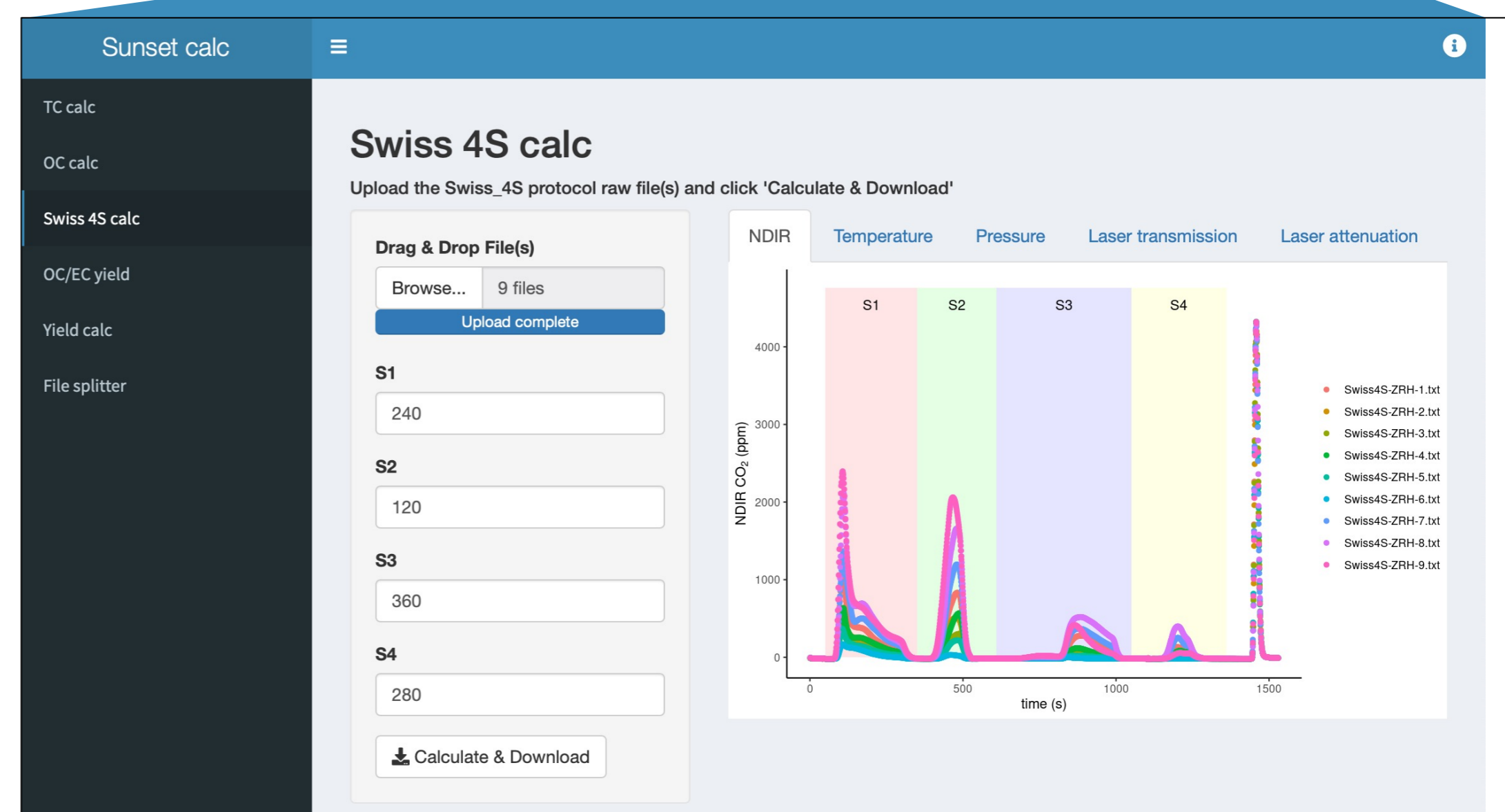
Fig. 6: Sunset-calc server deployment and user interface. The desired analysis is selected in the menu and the analyser raw data files are uploaded in the web interface. The calculation results are provided as a download. Changes to Sunset-calc in the repository are automatically deployed to the R server.
