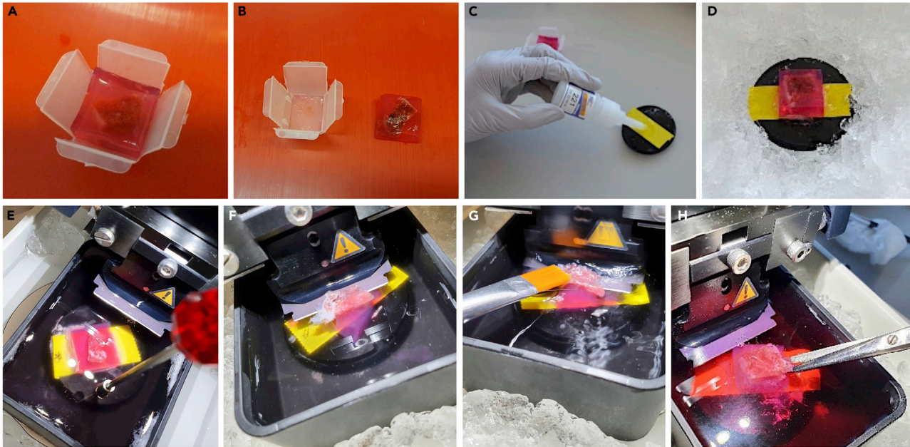
Figure 6. Sectioning process of embedded placenta pieces into precision-cut slices
