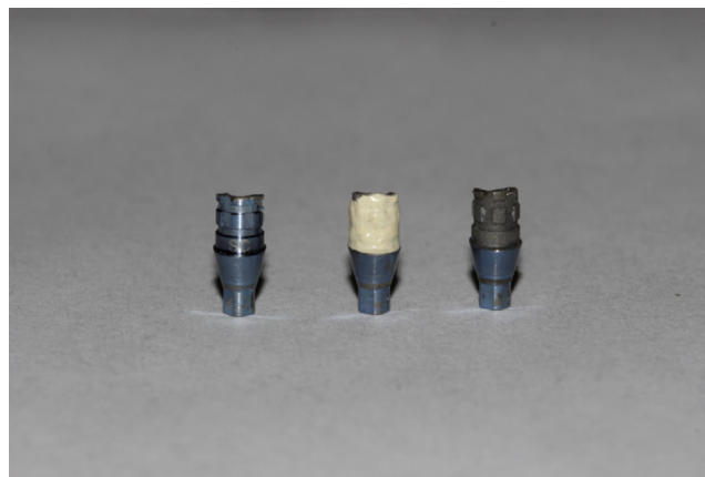
Figure 1. Interim abutments tested. Left control, center opaqued, right airborne-particle abraded.
