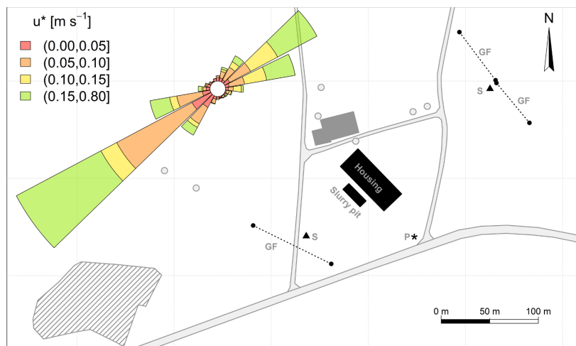
Fig. 1. Schematic overview of the measuring location with a wind rose. The wind rose indicates the frequency of occurrence of wind directions and the friction velocity u^* in each wind direction sector. The large black rectangle is the dairy cattle housing with the underground slurry pit on the southwest side. Filled black circles indicate positions of GasFinder (GF) sensors and retroreflectors with the dashed line representing the measuring path. The black triangles mark the position of the sonic anemometers (S). The inlet for the iTRM background measurements (P) is denoted as asterisk. Further, trees (grey circles), forest area (hatched polygon), a building (dark grey polygon) and the streets (light grey) are drawn.
